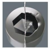
Hexagon screws can endure a problem because the contact surfaces delivering the power from conventional tool, transferred to the screw via very small surface areas. The consequence: the screw can become damaged (rounding out). Hex-Plus tools have a greater contact surface that prevents this from happening! At the same time, as much as 20 % more torque can be applied. Good to know: Hex-Plus tools fit into every standard hexagon socket screw!
