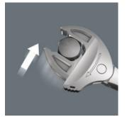
With its automatically and continuously gripping parallel jaws the Joker spanner 6004 covers all dimensions in the respective field of application. The tool automatically finds the required size when placed on the bolt or screw, no setting required.
