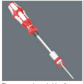
The screw gripper holds all screw profiles and sizes securely on the tool. Push the screw gripper onto the tip of the blade until the blade profile emerges from the rubber blade holder. Place the screw on the blade tip and fix it in the screw gripper. Pull the screw gripper further towards the handle until the two arms of the screw gripper rest on the screw head and are slightly spread.
