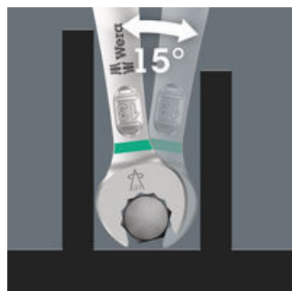
The Joker 6003 ring spanner with its special open end geometry - open end offset by 7.5° and the double hexagon profile - doubles the placement possibilities when repeatedly turning the wrench 180° around the longitudinal axis. Bolts and screw heads can be "accessed" every 15°. The Joker 6003 will automatically find the respective placement point after every turn.
