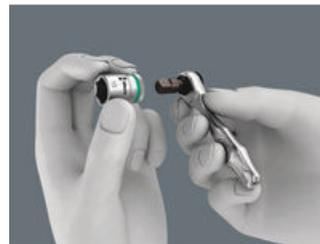
Bits and sockets. Bits can be connected directly. However, a holder can be connected first and then the bit can be attached to this. This then serves as an extension with a free-turning sleeve. An adaptor e.g. Wera 870/1 is needed for sockets - 1/4" hexagonal on a square drive (included in the Bit-Check and with the individual Zyklus Mini 1 in the set).
