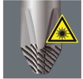
A precisely-focused laser creates a sharp-edged surface structure. Wera Lasertip "bites" itself into the screw head and prevents any slips out of the recess. It is available for screwdrivers for slotted, Phillips and Pozidriv screws.
