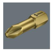
TH-Bits are hard bits with a torsion zone. Torsion bits absorb the damaging peak torque loads in the torsion zone. This prevents premature wear and enhances the service life of the bits.
