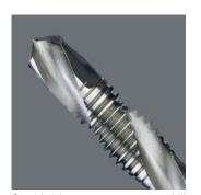
drill Combination bitsApplication: Corehole drilling, tapping and deburring in one operation1/4" drive suitable for holders as per DIN 3126-D 6.3 (ISO 1173)Hexagon shaft for very high torque transferHSS high speed steelFinely adjusted material elasticity for long service lifeExcellent centring propertiesStraightforward cuttingPerfect chip removalLow jamming riskPrecise return control
