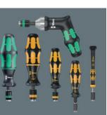
Wera torque screwdrivers. With a factory pre-set torque value set to the smallest scale value. For all applications, where the same constant torque and repeat accuracy are required. The torque can be changed with an extra tool within the measuring range (re-calibration kit can be ordered with the code number 05137003001). Afterwards you can check the set value using an off-the-shelf torque tester.
