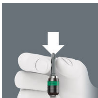
The bit can be pushed into the adaptor without moving the sleeve. The lock is activated automatically as soon as the bit is applied to the screw. Bits are held securely and wobble-free.
