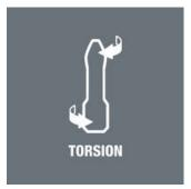
Torsion bits absorb the damaging peak torque loads in the torsion zone. This prevents premature wear and enhances the service life of the bits.
