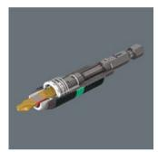
The effectiveness of the BiTorsion system comes from a combination of two shock-absorbing spring elements. Both, bits as well as holders have a cushioning torsion zone that diverts the kinetic energy away from the drive tip during peak loads.
