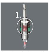
The torsion spring integrated into the unique BiTorsion holder absorbs lower levels of peak loads (Phase 1). Any overloading of this spring is effectively prevented by means of a supporting mechanism.
