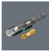
The optimally coordinated features of the torsion zones on the bit and holder permit a phased yield when under strain. The two-phase system prevents premature wear. Moreover, a long tool service life is also ensured by the hardness of the bits that matches the respective application.
