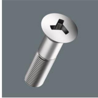
The TRI-WING® screwdriving system is mainly found in aviation and household technology (here e.g. on live components). The asymmetric arrangement of the three profile flanks prevents the use of anything other than the original tools. The high-precision Wera profile design ensures a secure fit of the tool in the head of the screw. The blades are manufactured out of bit material. The Wera know-how with regard to the hardening technology ensures a long service life of the tool.
