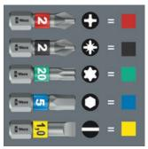
The "Take it easy" Bit-Checks have bits with a sleeve which from its colour (e.g. red = Phillips) and size designation - make it simple to access the right bit quickly. Bit-Check 6 TX Impaktor 1, 6 pieces
