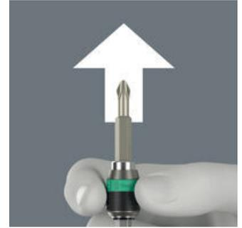
Simply push the sleeve forward to change the bit. The spring mechanism lifts the bit off the magnet and unlocks the tool. The rapid-out function makes it easy to remove even the smallest bits without extra tools.
