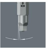
V bits have a conical profile. The clamping forces thus resulting hold Robertson screws securely on the tip of the tool. Ideal for screwdriving at difficult-to-access places.
