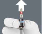
Simply push the sleeve forward to change the bit. The spring mechanism lifts the bit off the magnet and unlocks the tool. The bit can be easily removed. The rapid-out function makes it easy to remove even the smallest bits without extra tools.
