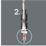
Higher peak loads are minimised through the torsion effect of the bit shaft (Phase 2).
