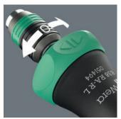
Switching the screwdriving direction is intuitive: Turn the ring switch clockwise for clockwise screwdriving, turn it counterclockwise for counterclockwise screwdriving.
