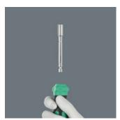
By pressing the locking sleeve again with more force, the loosening mechanism is released by a clearly audible and tactile overcoming of the locking resistance. The telescopic blade can be removed and inserted into electrical screwdrivers as a bit adapter.
