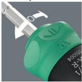
Intuitive switching of the ratchet mechanism. Turn the switch clockwise clockwise for screwdriving; it turn counterclockwise for counterclockwise screwdriving. Use position 0 to deactivate the ratchet mechanism for precise working.
