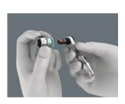
1/4" sockets can also be used with the Zyklop Mini bit ratchet by connecting the 870/1 adapter (1/4" hexagon to 1/4" square head).
