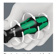
The hard materials used for the handle ensure rapid hand repositioning without any danger of the skin "sticking" to the handle. The surrounding hard zones with large diameters glide like wheels through the hand.
