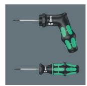
Wera torque-indicators have been factory pre-set to values recommended by leading carbide manufacturers. tool These tightening values relate specifically to the size of the TORX®, TORX PLUS® or hexagon socket screw. Torque indicators ensure safe and screw easy loosening of connections. Precision :  $\pm$  10 %
