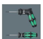
Wera torque-indicators have been factory pre-set to values recommended by leading carbide manufacturers. tool These tightening values relate specifically to the size of the TORX®, TORX PLUS® or hexagon socket screw. Torque indicators ensure safe and screw easy loosening of connections. Precision: ± 10 %
