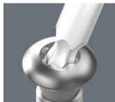
The spherical drive profile means that it is possible to swivel the axis of the tool to that of the screw, and therefore enable angled, "around-the-corner" screwdriving jobs.
