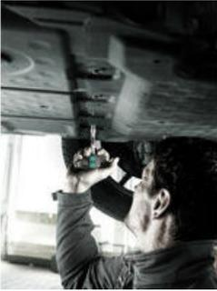
The 411 A RA T-handle is suitable for 1/4" sockets. The sockets are securely locked via the ball.
