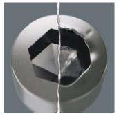
Hexagon screws can endure a problem because the contact surfaces delivering the power from conventional tool, the is transferred to the screw via very small surface areas. The consequence: the screw can become damaged (rounding out). Hex-Plus tools have a greater contact surface that prevents this from happening! At the same time, as much as 20 % more torque can be applied. Good to know: Hex-Plus tools fit into every standard hexagon socket screw!
