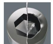
Hexagon screws can endure a problem because the contact surfaces delivering the power from conventional tool, is transferred to the screw via very small surface areas. The consequence: the screw can become damaged (rounding out). Hex-Plus tools have a greater contact surface that prevents this from happening! At the same time, as much as 20 % more torque can be applied. Good to know: Hex-Plus tools fit into every standard hexagon socket screw!
