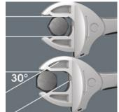
Thanks to the corner-width rectangular prisms in both jaws of the double spanner, a return angle of only 30° can be achieved.
