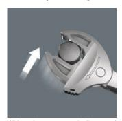
With its automatically and continuously gripping parallel jaws, the Joker 6006 double spanner covers all dimensions within the potential operative range. The tool finds the required size by itself when attaching it to the bolt or screw.
