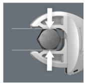
The parallel, smooth jaws of the Joker 6006 double spanner offer a seating stress and can thus prevent the nut or screw head from rounding, which can occur when power is transmitted over corners.
