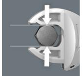
The parallel, smooth jaws of the 7870 Joker offer a seating stress and can thus prevent the nut or screw head from rounding, which can occur when power is transmitted over corners.
