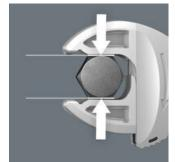
The parallel, smooth jaws of the 7880 Joker offer a seating stress and can thus prevent the nut or screw head from rounding, which can occur when power is transmitted over corners.
