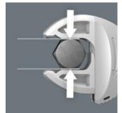
The parallel, smooth jaws of the Joker 7880 offer a seating stress and can thus prevent the nut or screw head from rounding, which can occur when power is transmitted over corners.
