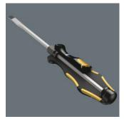
Wera makes its Kraftform handles from several materials with different properties. The core is made from a hardwearing plastic that holds the blade securely even when subjected to great forces. The yellow soft zones of the external mantle consist of a softer material with more friction resistance for high torque transfer. The black areas with a harder surface prevent the hand from sticking to the handle enabling you to adjust your grip more quickly. Kraftform Plus – Series 900
