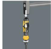
With the impact wrench function switched on, the hammer blow impulse is converted into a rotary movement with a loosening moment of up to 25 Nm. Power transmission without loss via a pound-thru blade.
