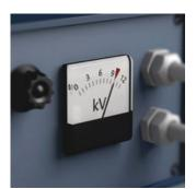
Testing the tool for dielectric strength at 10,000 volt gives the user the peace of mind that their tool has been tested for its most important property, insulation. Wera VDE tools are subjected to this test piece by piece which guarantees safe working at up to 1,000 volt.
