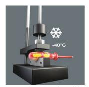
Impact strength tested at -40°C, guaranteeing safety even under extreme conditions.
