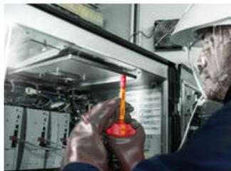
One 410 i VDE A RA T-handle adapter screwdriver with ratchet functionality for 1/4" sockets and 1/4" bit sockets
