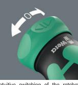
Intuitive switching of the ratchet mechanism. Turn the switch clockwise clockwise for screwdriving; it turn counterclockwise for counterclockwise screwdriving. Use position 0 to deactivate the ratchet mechanism for precise workina.
