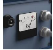
Our screwdrivers are tested for dielectric strength under a 10,000 volt load to make sure that their most important property, their insulation, has been exhaustively tested. Each individual Wera VDE screwdriver is subjected to this test to guarantee safe working up to 1,000 volts. VDE interchangeable blades 154 mm long
